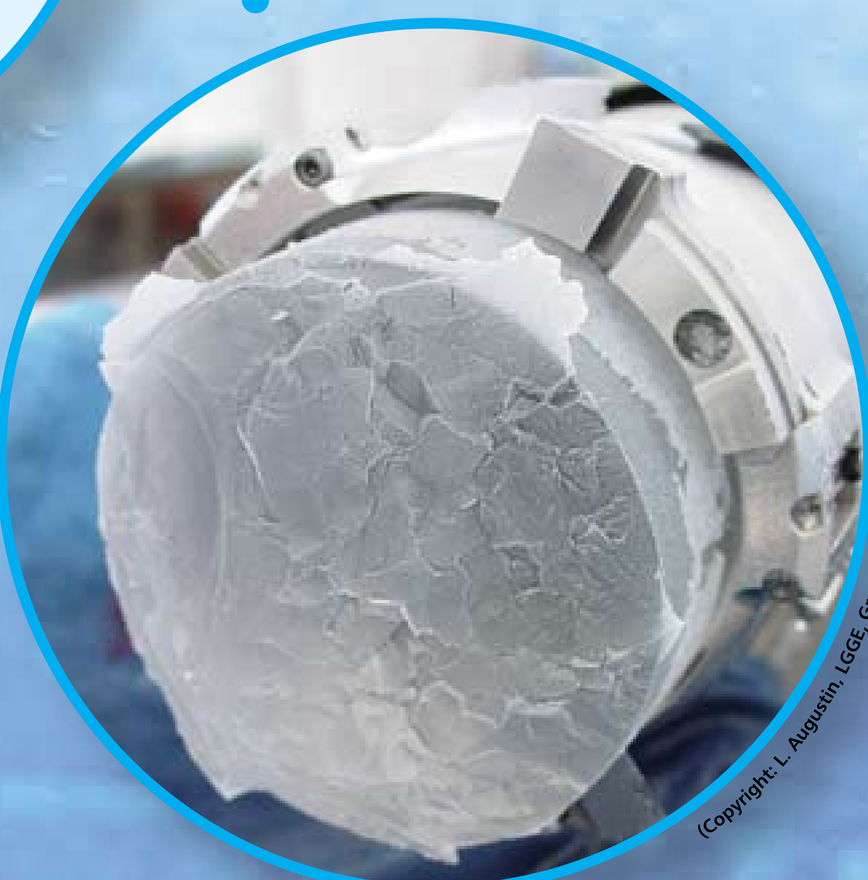
Drill head and ice core from a depth of 2,874 m from Dome Concordia Station, drilled on November 30, 2002. The age of the ice is about 491,000 years. Drill head and cutters were designed and constructed by Henry Ruffli (University of Bern, Switzerland).
