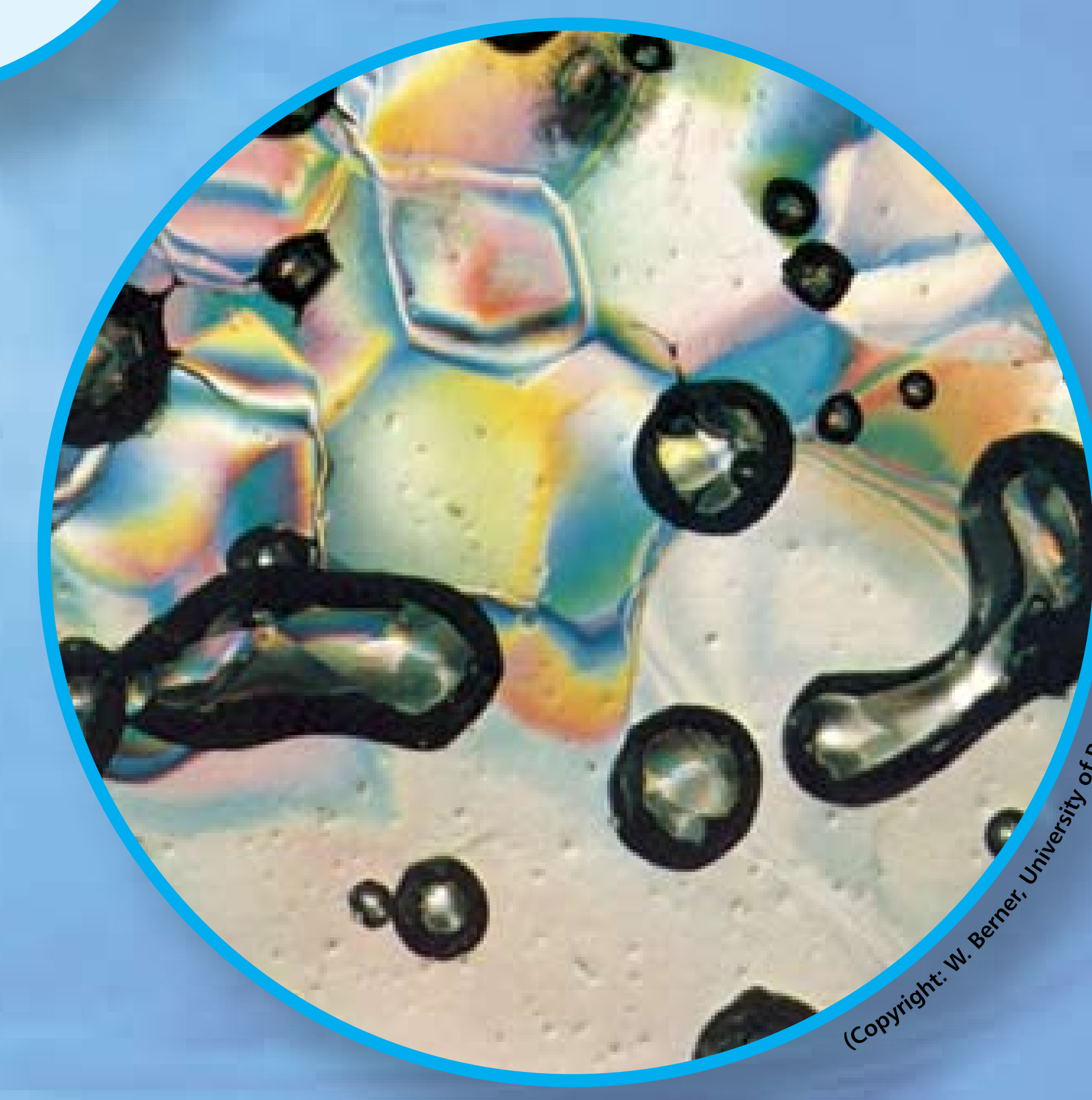
Thin cut of a polar ice sample illuminated through two polarizing filters. Grain boundaries appear in rainbow colours; the gas bubbles enclosed in the ice are dark. The diameter of the bubbles ranges from 1 to 3 mm. The analysis of the gas composition in these bubbles permits the reconstruction of greenhouse gas concentrations (CO 2 , CH 4 , and N 2 O) of the past 900,000 years.
